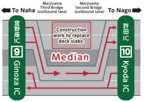
The four inbound and outbound lanes will be reduced to two lanes (two-way traffic) during deck slab replacement.
